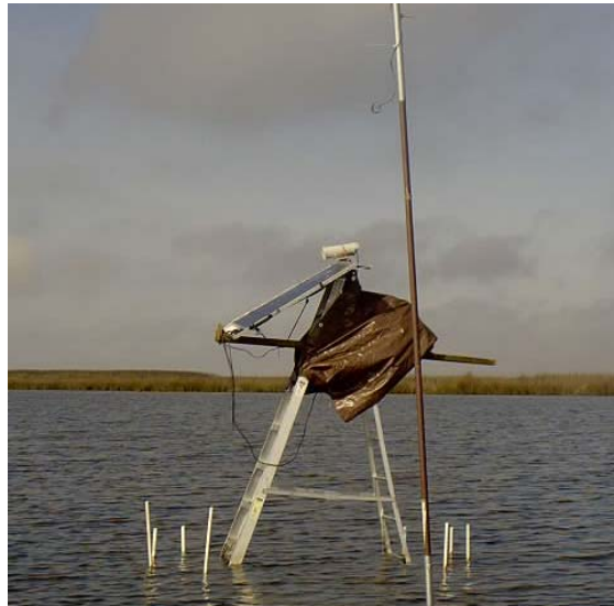
Figure 24. Camera system (camera, solar panel, VCR, and timer) deployed in an untterraced pond in Rockefeller's Unit 4, winter of 2005, Chenier Plain, Louisiana. Tripod made of ten-foot ladder with attached 6 ft. shelf. Lightning rod made of copper and aluminum pipe is in foreground.
